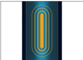
The State LED blinks in orange, for 90 seconds, and the cleaning process proceeds automatically.
