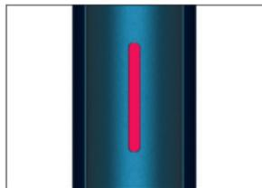
State LED lights in red for 3 seconds and vibration occurs 3 times, simultaneously. The battery is insufficient. Charge the device.
