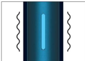
When the device is completely reset, the State LED lights in ice blue for 1 second, and vibration occurs twice, simultaneously.
