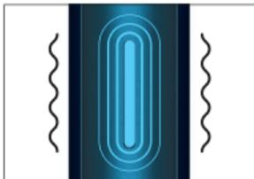
After 2 seconds, the State LED blinks in ice blue, and vibration occurs simultaneously.
