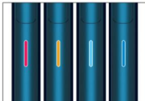
While the device wakes up, the Status LED blinks twice in red, orange, ice blue and blue, sequentially.
