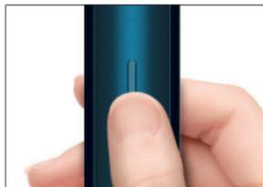
Press the Button for 8 seconds, even if vibration occurs within 2 seconds.
