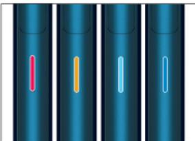
The device is reset, and the State LED blinks twice in red, orange, ice blue and blue, sequentially.
