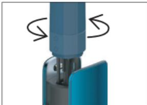
Insert the Cleaning Wiper into the device and clean the device by spinning the Cleaning Wiper.
