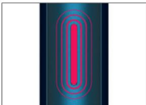
State LED blinks in red 5 times. The device is malfunctioning. Reset the device.
