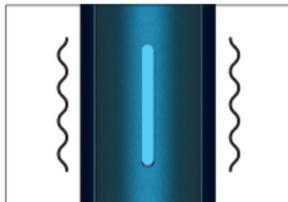
When the preheating process ends, the State LED lights come on, and vibration occurs simultaneously. This means that the preheating process has ended, and the stick is ready for use.
