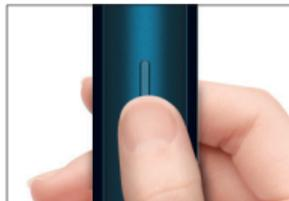
The device is in the sleep mode and does not operate unless activated for your first use. To wake up the device press the Button for 2 seconds or connect the charger to the charging port.
