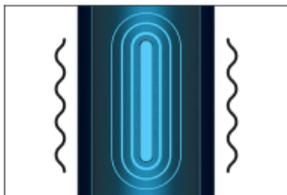
To signal the last 30 seconds of the session or the last 3 puffs, whichever comes first, the device will vibrate once and the State LED will blink in ice blue until the end of the session.
